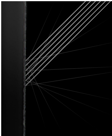
Light scattering on nano-texture cover glass
