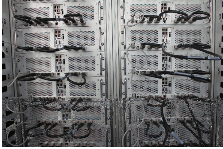
Figure 4: Close-up view of the Janus II machine installed at BIFI (Zaragoza). The installation has 16 Janus II boxes (12 are visible in the picture). The cables supporting the data-links in the z direction are mounted in loop-back mode for test purposes.
