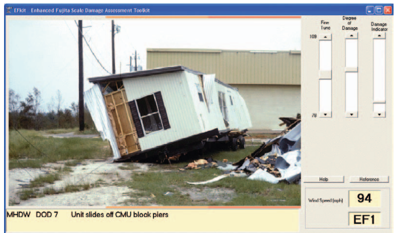
FIG. 1. Screen example of EFkit PC software used in many NWS damage surveys as of this writing. Defaults of both values and photographic example are shown for a double-wide mobile home (MHDW; per Table 1) at DoD 7. Users can select the DI (right) and DoD (middle) while sliding the “fine tune” bar up and down to allow for some subjectively assessed leeway in rating: for example, reducing the wind speed if much weaker or no adjacent damage is evident.
