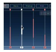
When the highpass filter cutoff frequency value is lower than that of the lowpass cutoff frequency, only one line is shown. This line represents the frequency band that passes through the filters—in other words, the filters act as a bandpass filter. In this configuration, the two filters operate in series which means the tap passes through one filter first, then the other.
