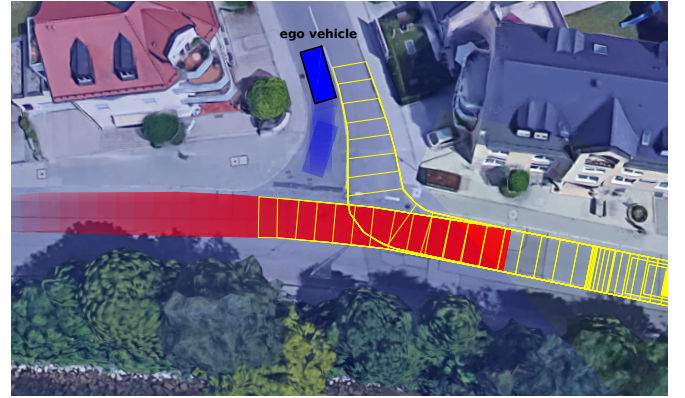
Figure 1: Dangerous intersection with occlusions. Yellow: The obstacle is occluded by a container, such that it and its reachable set is not known to the ego vehicle. Red: We can over-approximate the reachable set of possibly hidden vehicles and adapt the ego trajectory (transparent blue) to still guarantee safety. Imagery © 2018 Google, Map data © 2018 GeoBasis-DE/BKG.
