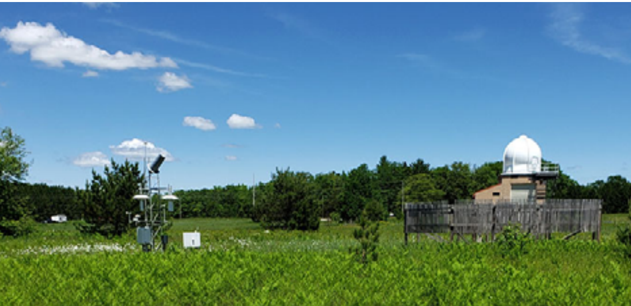
US Climate Reference Network Station in Gaylord, Michigan. The precipitation gauge at right, is surrounded by fencing. Image credit: NOAA
