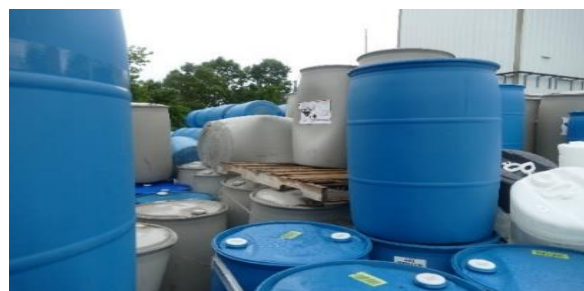
Chemical drums improperly stacked and some drums under duress.
