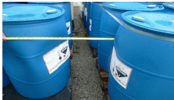
Insufficient aisle space between chemical drums.
